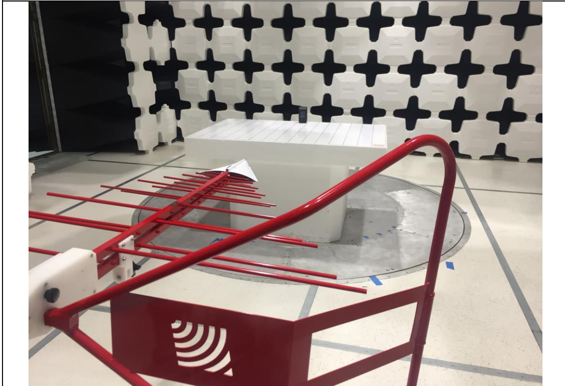
Radiated Emissions Below 1GHz setup – MMK200
