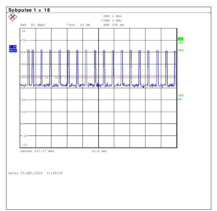
Test Data: 100 ms Number of Pulses Plot
