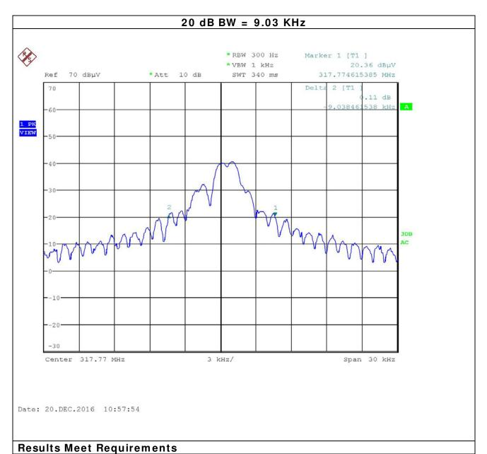
Test Data: 20 dB Occupied Bandwidth Plot
