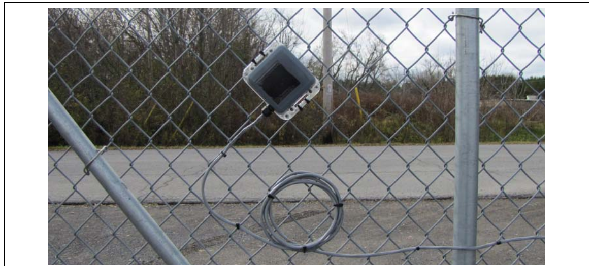
Figure 45: Solar powered Wireless Gate Sensor with magnetic gate contact
