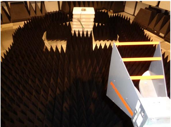
Note: Additionally the EUT was scanned at 1.5 meter height on top
