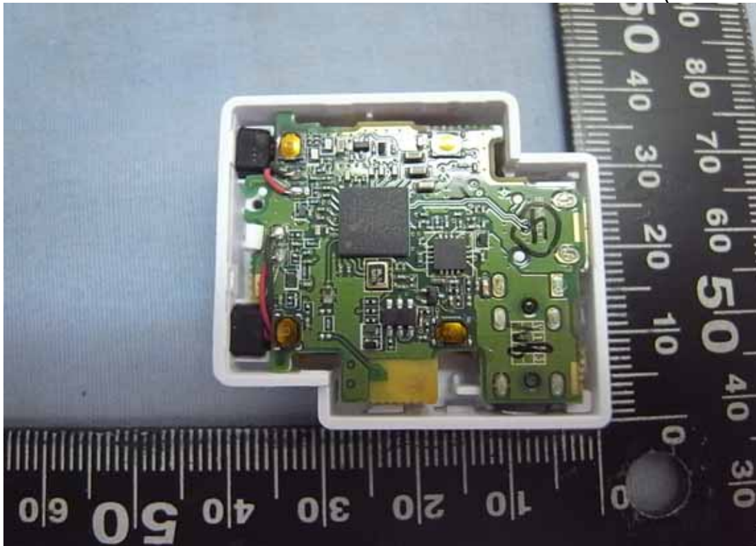
Figure 9 Internal View (Removed Cover)
