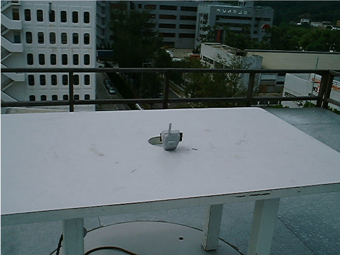
Measurement of Radiated Emission Test Set Up
