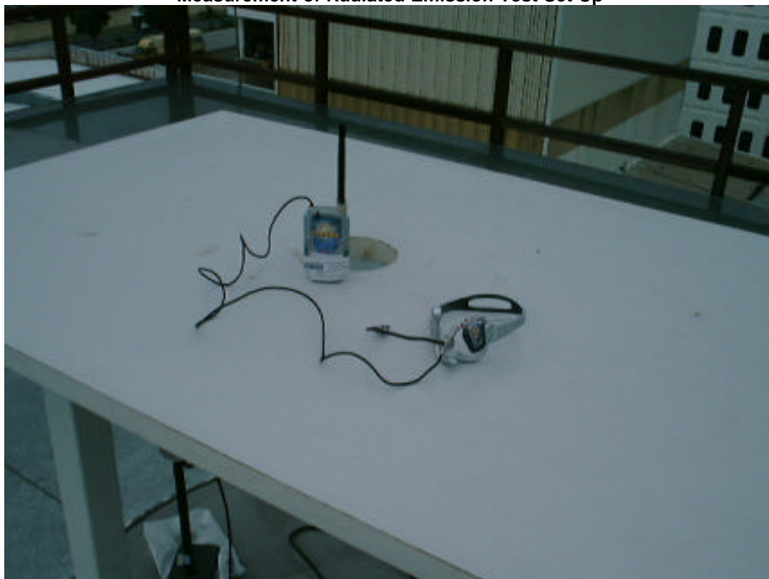
Measurement of Radiated Emission Test Set Up
