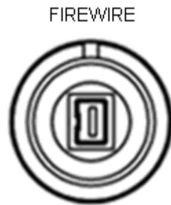
Figure 4-11: Firewire Input Connector (Optional) (Contact Nucomm for availability of this option.)
