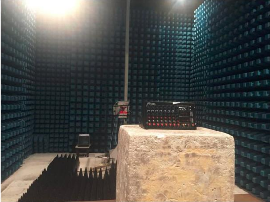
Description: Radiated Emission Test Setup for 1~18GHz
