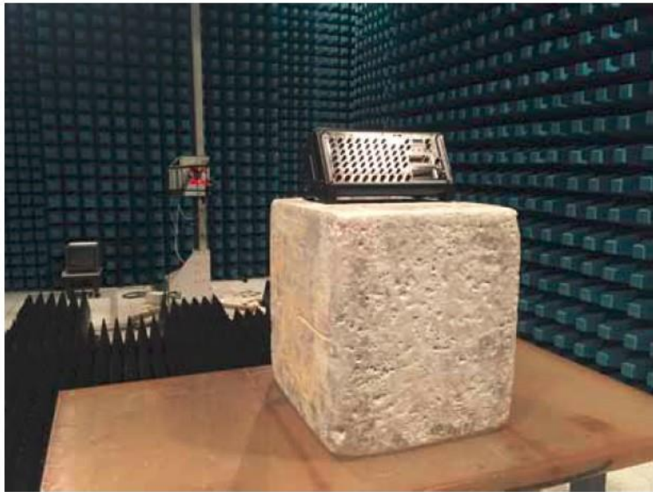
Description: Radiated Emission Test Setup for 1~18GHz
