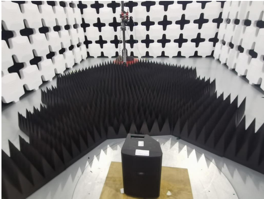
PVX p10 Radiated Emission test Above 1GHz
