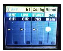
Fig. 2 Main (Master) Channel Gain (Default)
