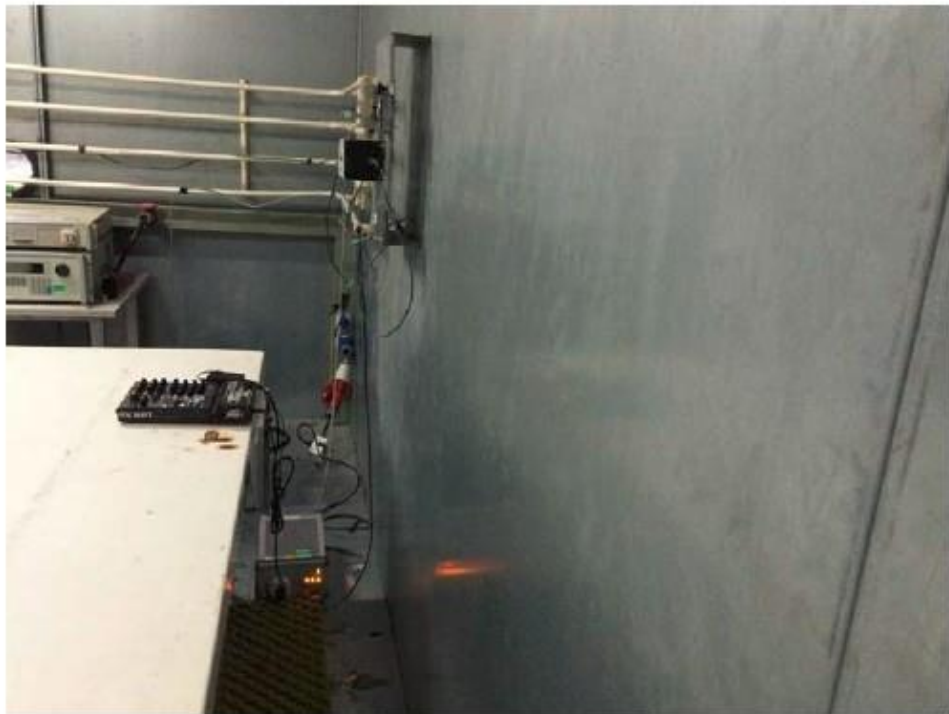
Description: Conducted Emission Test Setup
