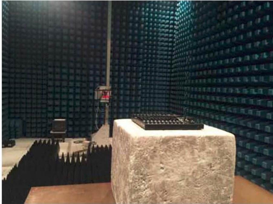
Description: Radiated Emission Test Setup for 1~18GHz
