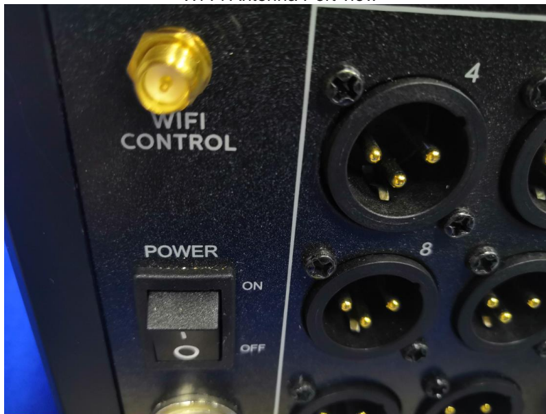
Wi-Fi Antenna Port view
