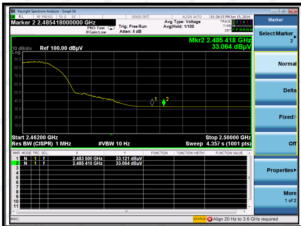
(Plot B2: Channel = 11 AVG @ 802.11b)
