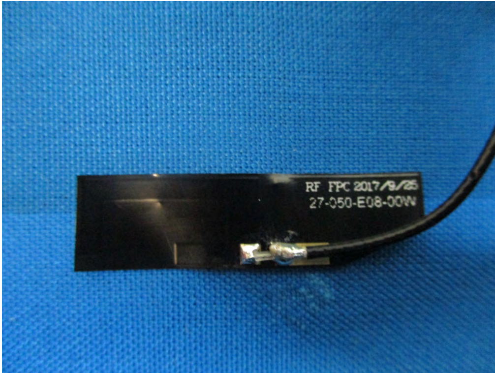
FPC Antenna – View
