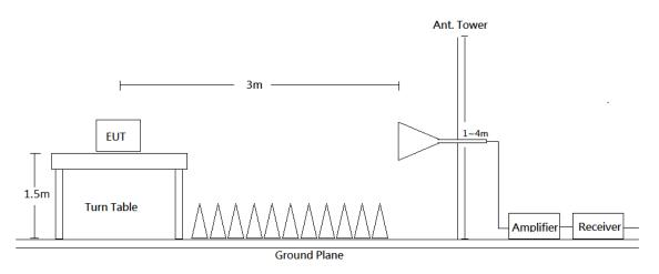
The radiated emission tests were performed in the 3 meters test site, using the setup accordance with the ANSI C63.10-2013. The specification used was the FCC 15.209, and FCC 15.249 limits.
