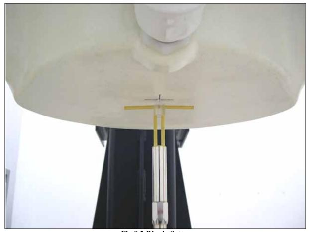
Fig 8.2 Dipole Setup
