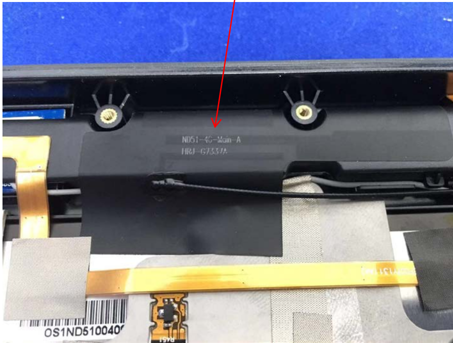
LTE/WCDMA Main Antenna
