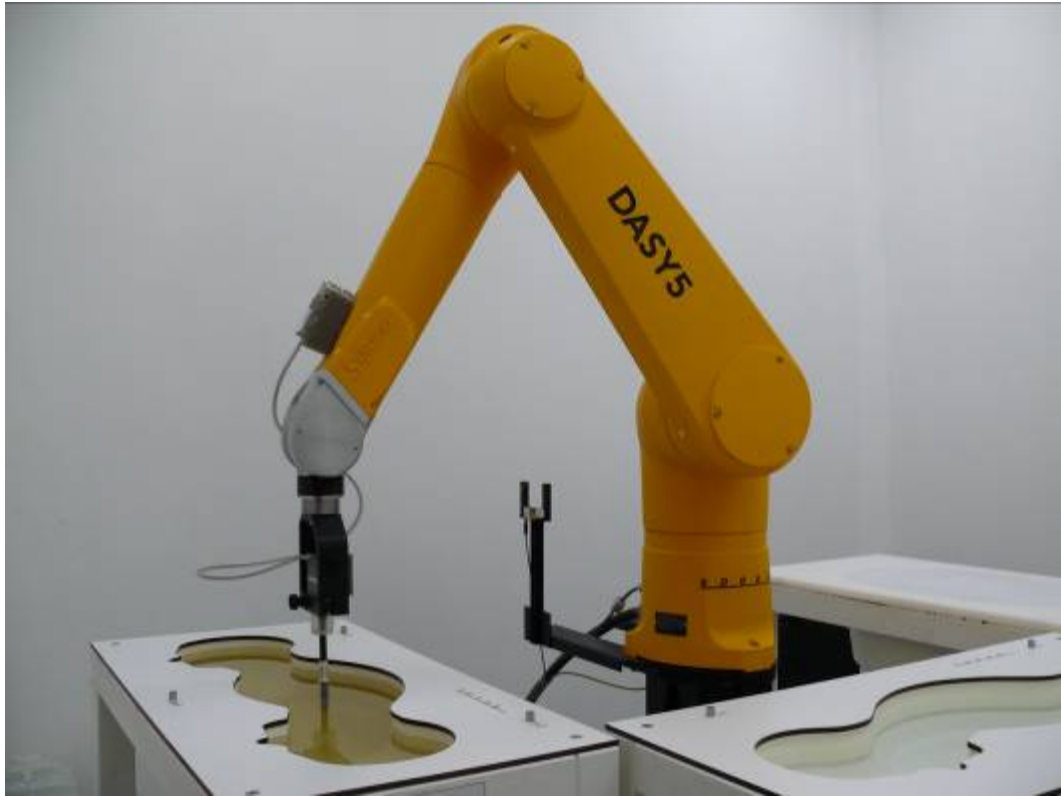
Picture 1: Specific Absorption Rate Test Layout
