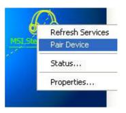
You shall be prompted to enter Bluetooth passkey, enter default passkey **0000**, and then click **OK** to complete pairing process. The LED indicator of FS310 shall light up un-interrupted showing pairing mode.
