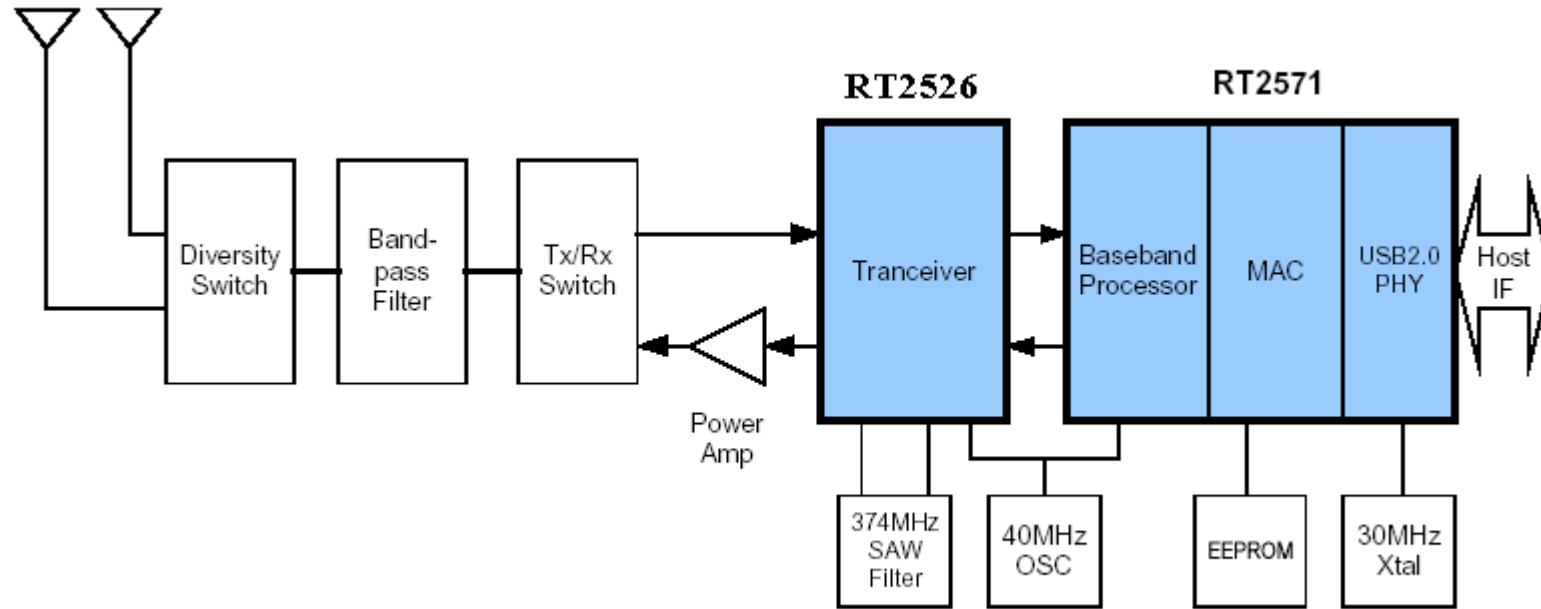
U31 MAC controller and baseband processor (RT2571) → Determine the modulation type (DBPSK、DQPSK、CCK、OFDM) → send out Tx I & Tx Q signal → U9 Radio IC (RT2526) → Mixed Tx I & Tx Q signal with RF local signal (2412~2484MHz) → Sent out transmission signal → U5 Power Amplifier (BAP2101) to amplify the signal → BPF → U6 Tx/Rx switch → U46 antenna select switch → Dipole Antenna transmission signal is sent out from single antenna.
