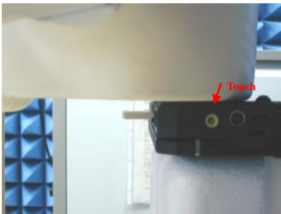
Fig.4 Photograph of the Bottom of the Pc is paralleled and at a distance of 0.0 cm from the base of the phantom.
