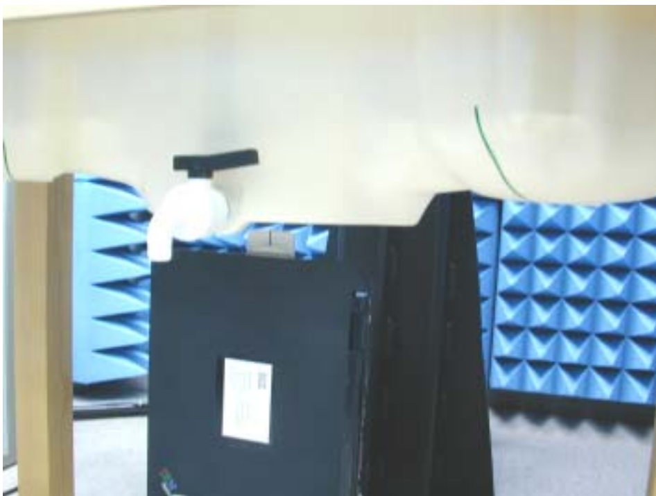
Fig.6 Edge of the PC at 90° and at a distance of 1.5 cm from the base of the phantom.
