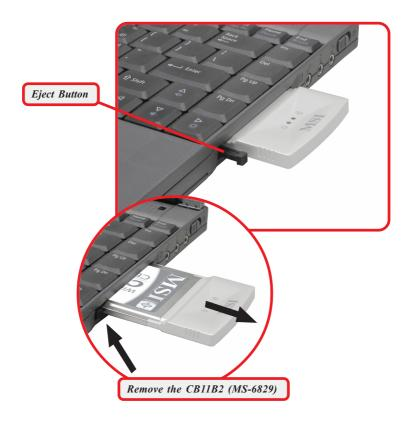
Before removing the CB11B2 (MS-6829), you should stop the device in Windows operating system.
