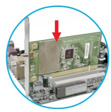
**Step 3.** Replace the computer cover after securing the PC11B2 (MS-6828) with a bracket screw.
