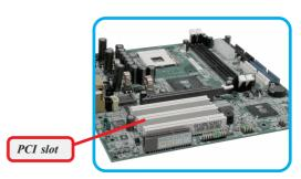
**Step 2.** Put the PC11B2 (MS-6828) directly over the PCI slot and press it into the slot firmly.
