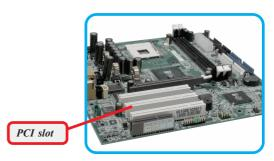
**Step 2.** Put the PC54G (MS-6825) directly over the PCI slot and press it into the slot firmly.
