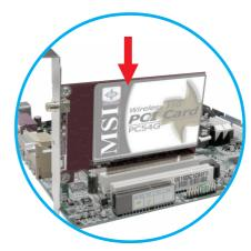
**Step 3.** Replace the computer cover after securing the PC54G (MS-6825) with a bracket screw.
