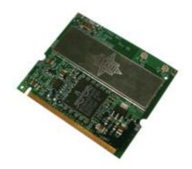
MSI-6804 IEEE 802.11b Mini PCI is an embedded solution that complies with IEEE 802.11b standard and provides 11 Mbps data rate. The small form factor and light weight design are suitable for mobile devices, desktop, laptop and Internet Appliance with Mini-PCI slot. Integrated with it, the device can easily share a broadband connection, files and printers over the network wirelessly. In addition, with 64-/128-bit Privacy Key and IEEE 802.11i TKP, network connection is highly secured.
