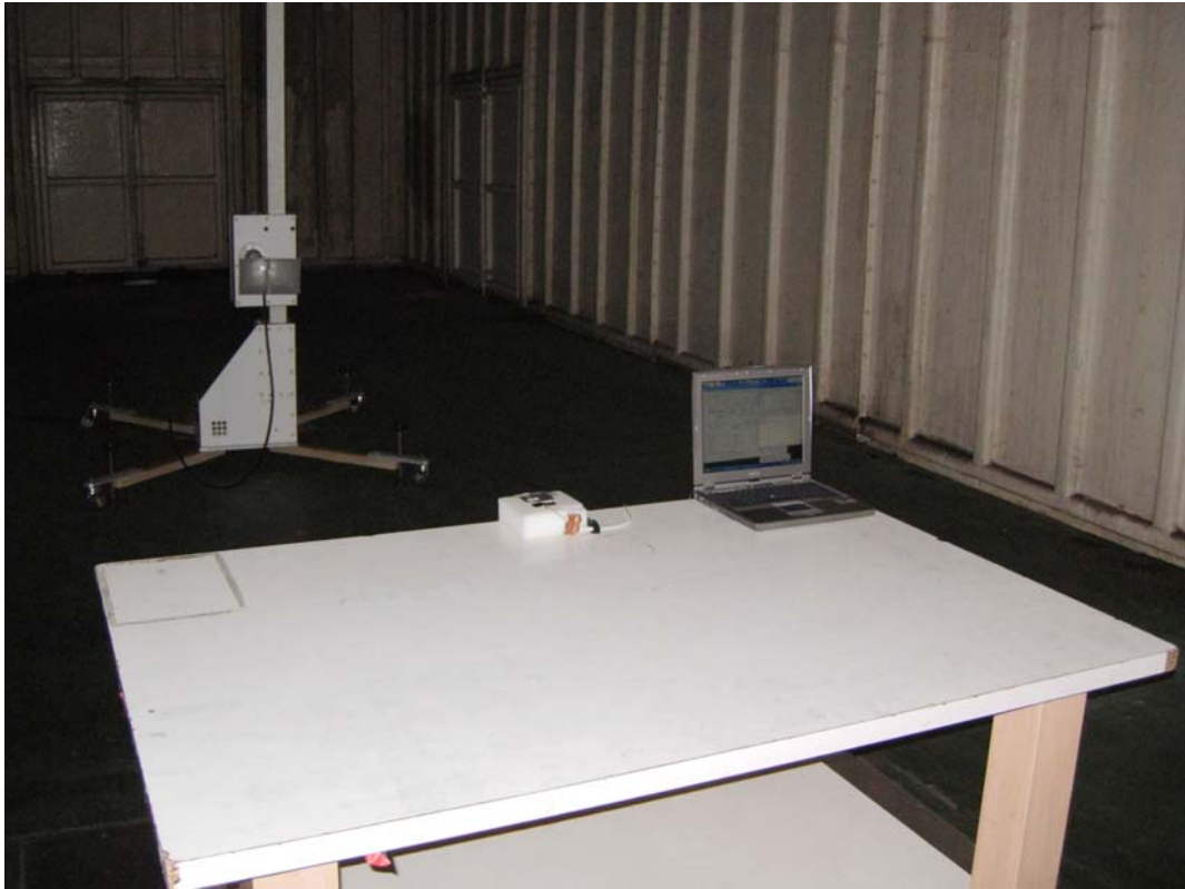
Back View of Radiated Test (Horn) - Shielding C (X-axis)
