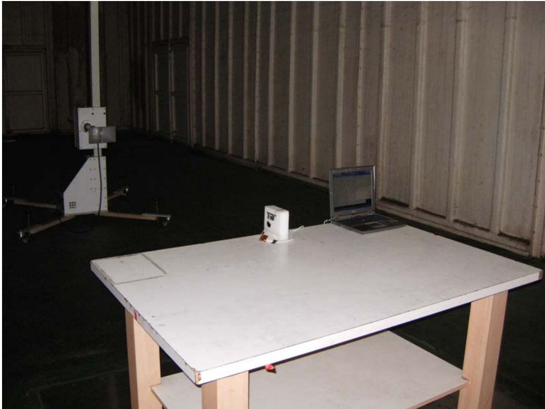
Back View of Radiated Test (Horn) - Shielding B (Z-axis)
