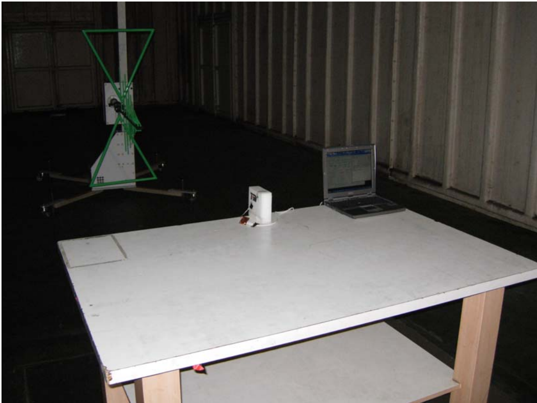
Back View of Radiated Test - Shielding B (Z-axis)
