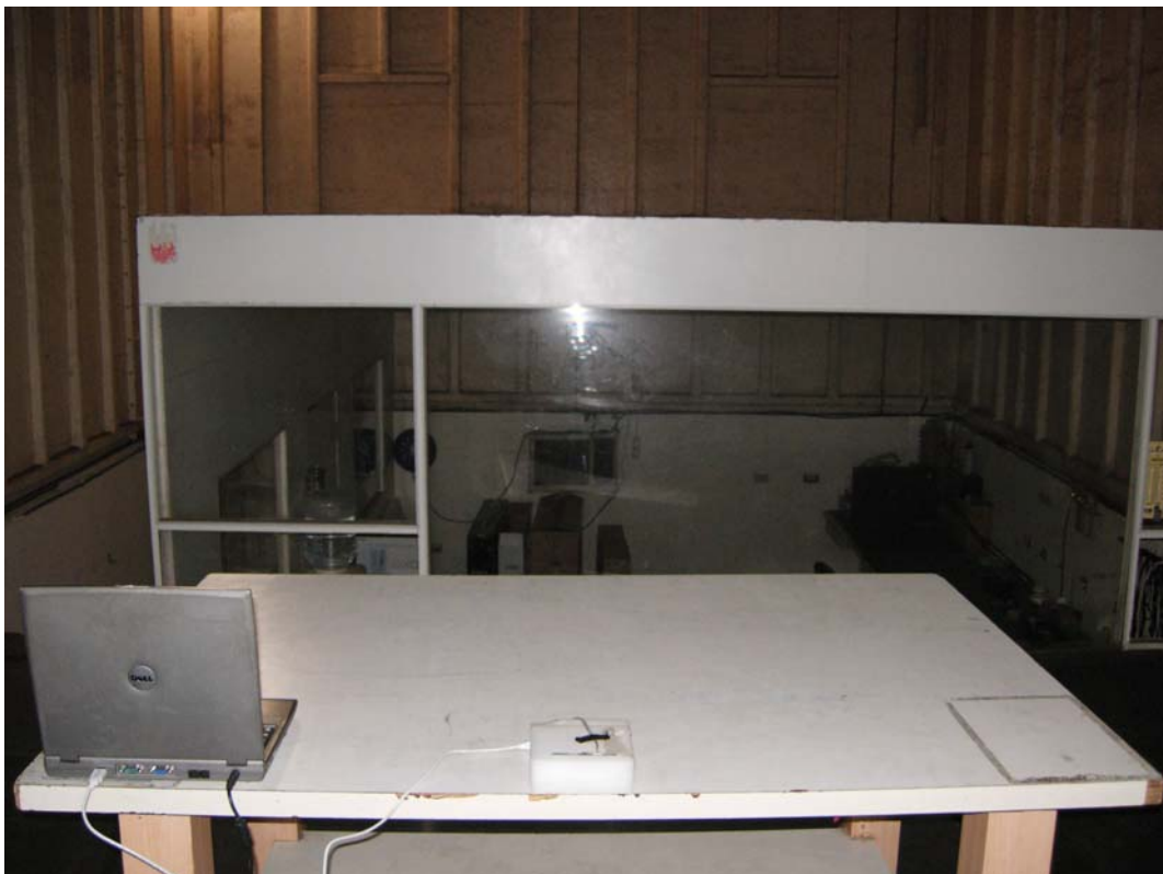
Back View of Radiated Test - Shielding A (X-axis)
