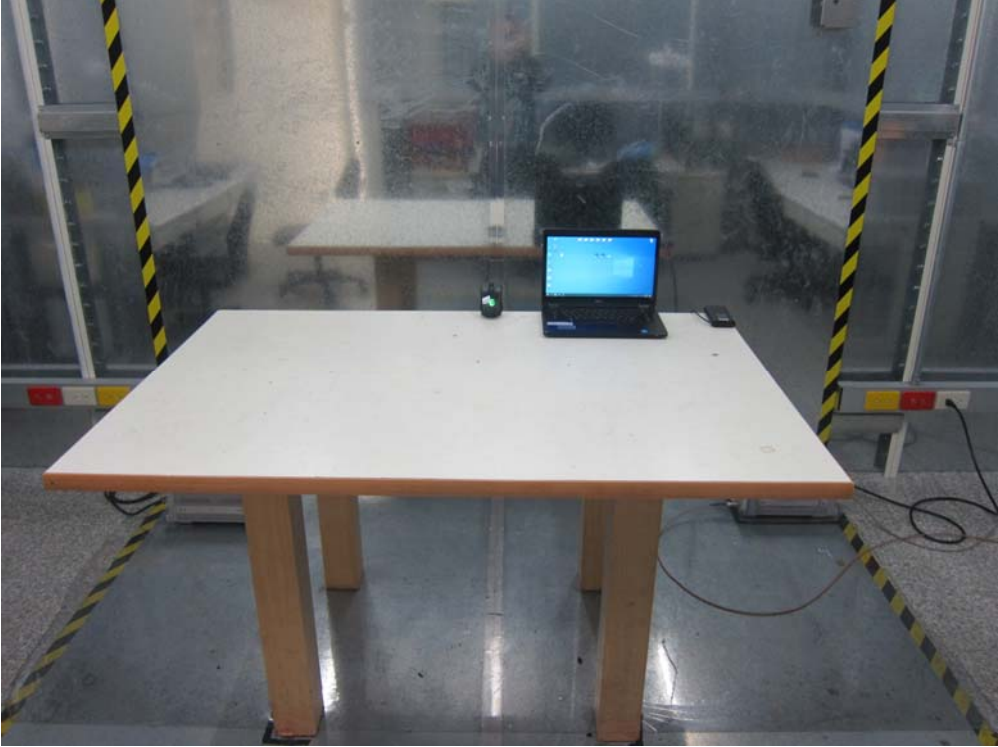
Front View of Conducted Test - Charge Mode
