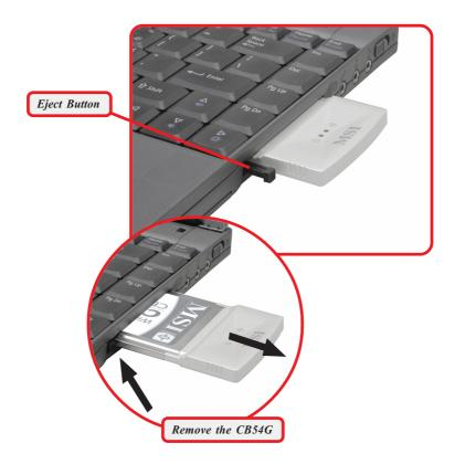
Before removing the CB54G, you should stop the device in Windows operating system.
