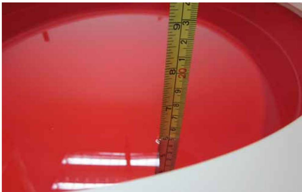
Figure 4.4: Liquid depth in the Flat Phantom
