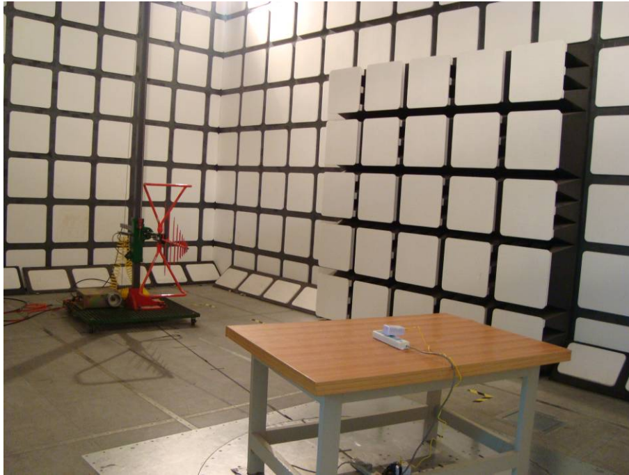
Below 1GHz: Spurious Radiated Emissions - Rear View
