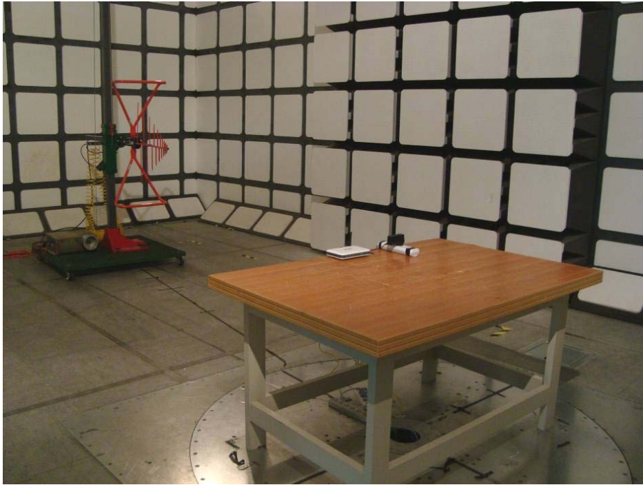
Below 1 GHz: Spurious Radiated Emissions - Rear View
