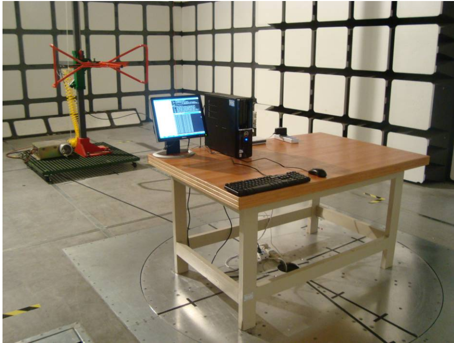
Below 1GHz: Spurious Radiated Emissions - Front View
