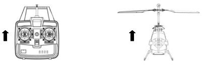
When throttle is pushed up, rotor speed increases and Helex lifts up.
