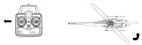
When rudder is moved to the left, nose of Helex turns left.
