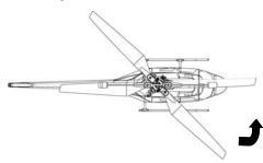
When rudder is moved to the left, nose of Helex turns left.
