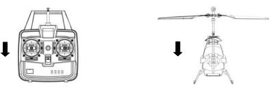
When throttle is pushed down, rotor speed reduces and Helex descends.
