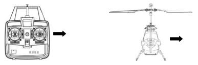
When aileron is moved to the right, swash plate should also tilt and Helex moves to the right.
