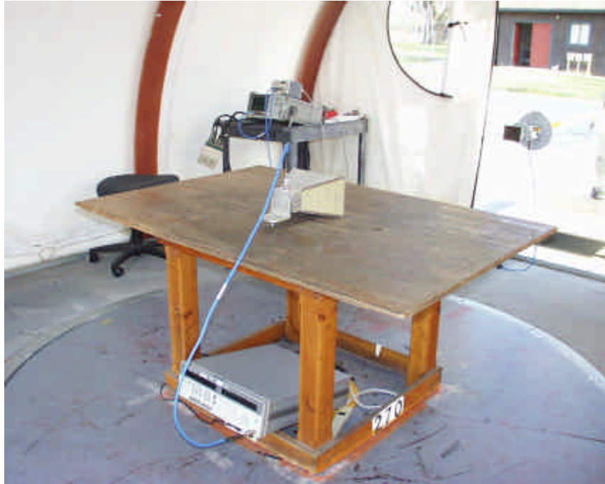
18 – 20 GHz Substitution Method Setup
