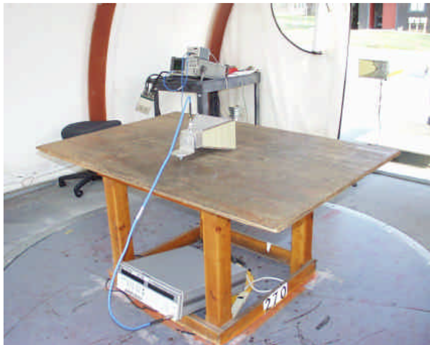
1 – 18 GHz Substitution Method Setup
