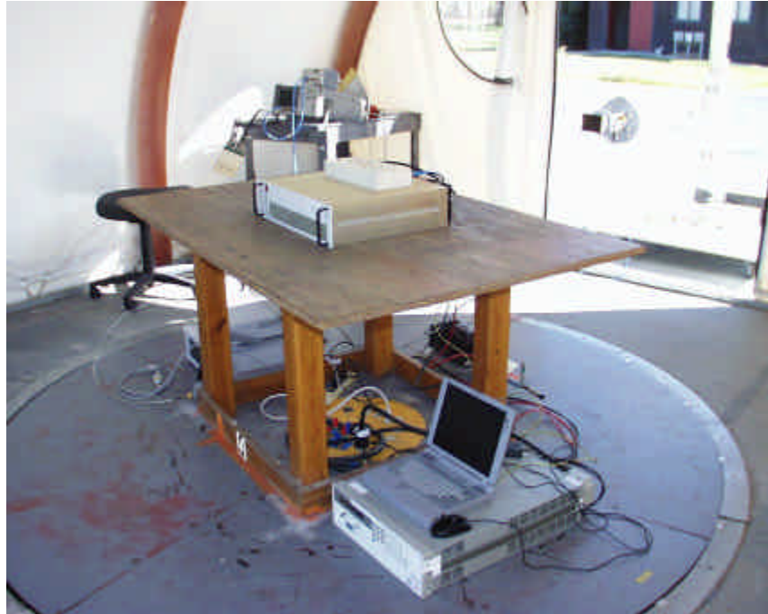
18 – 20 GHz Radiated Emission Setup
