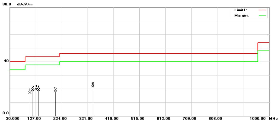
**BLE(1M) Mode** (Pre-scan with three orthogonal axis, and worse case as X axis.)**Horizontal** (worst case is high channel)
