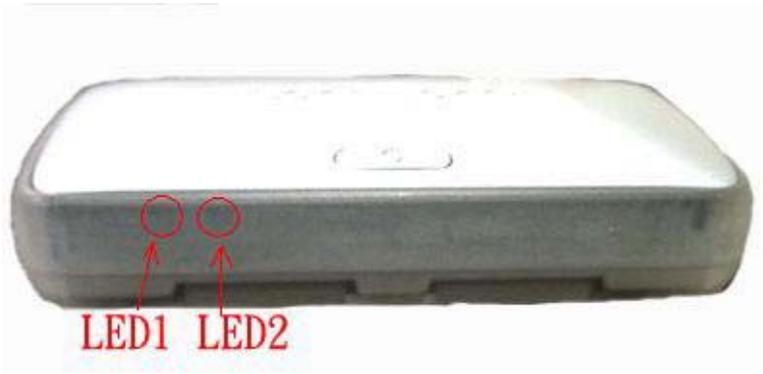
The Bluetooth GPS has two LED light which each has two colors. One is GPS & Charge status LED, that is named LED 2, and the other is Bluetooth & low power status LED, that is named LED 1. The status table of LED shows as follows:
