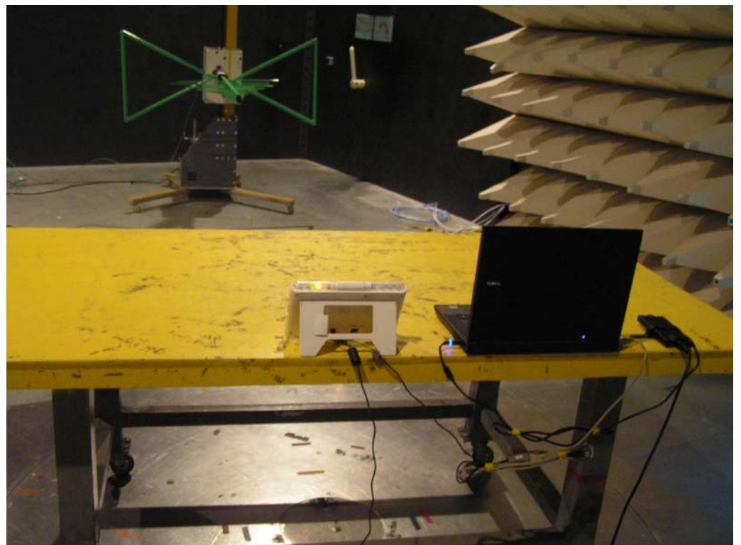
**For radiated emissions above 1GHz****FRONT VIEW**
