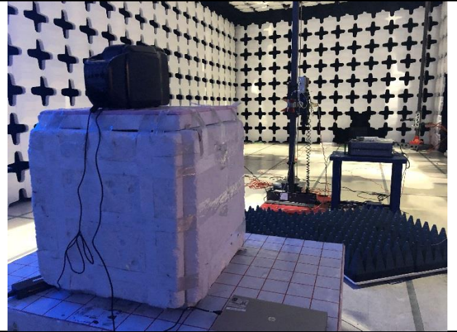
Radiated Emissions (>1GHz) – Rear View
