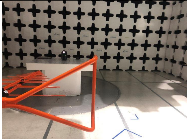
Radiated Emissions (<1GHz) – Front View
