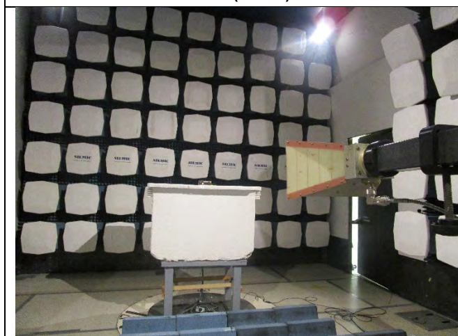
Radiated Emissions (>1GHz) – Front View
