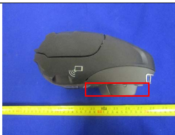
Extended battery installed
