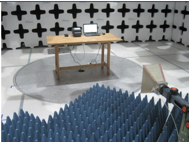
Test setup at 3 meter distance (>1GHz) - Front
