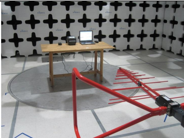
Test setup at 3 meter distance (<1GHz) - Front
