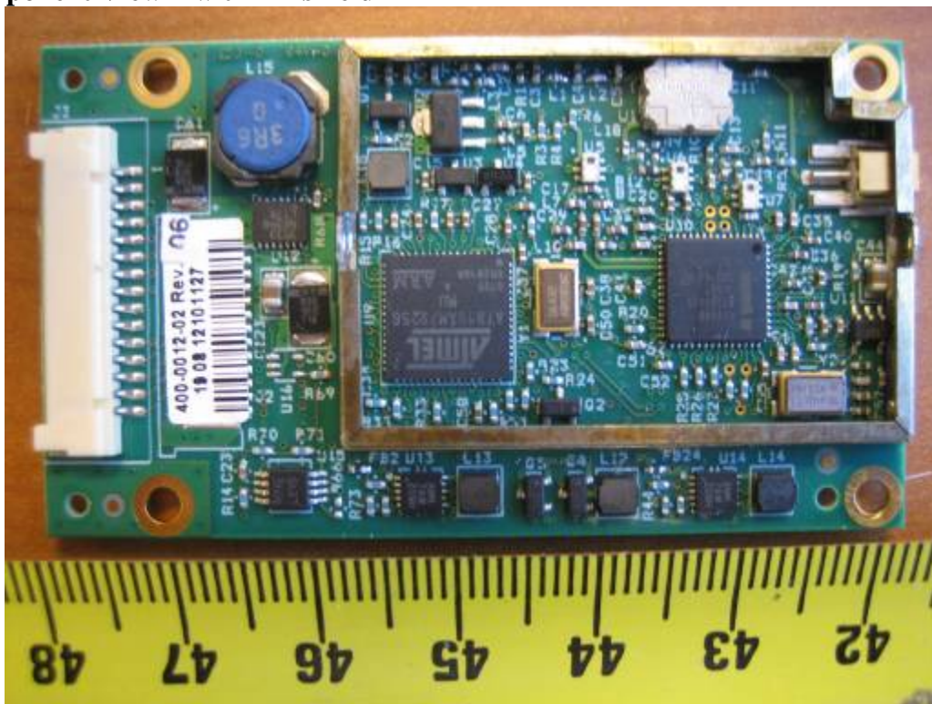
Component View-1 with RF shield
