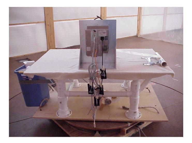
Company: Zebra Technologies Corporation Product: R110PAX4 FCC ID#: I28RFID-R110PAX02 Date: 1/7/2005 Photo Description: Radiated Testing – Front of EUT
