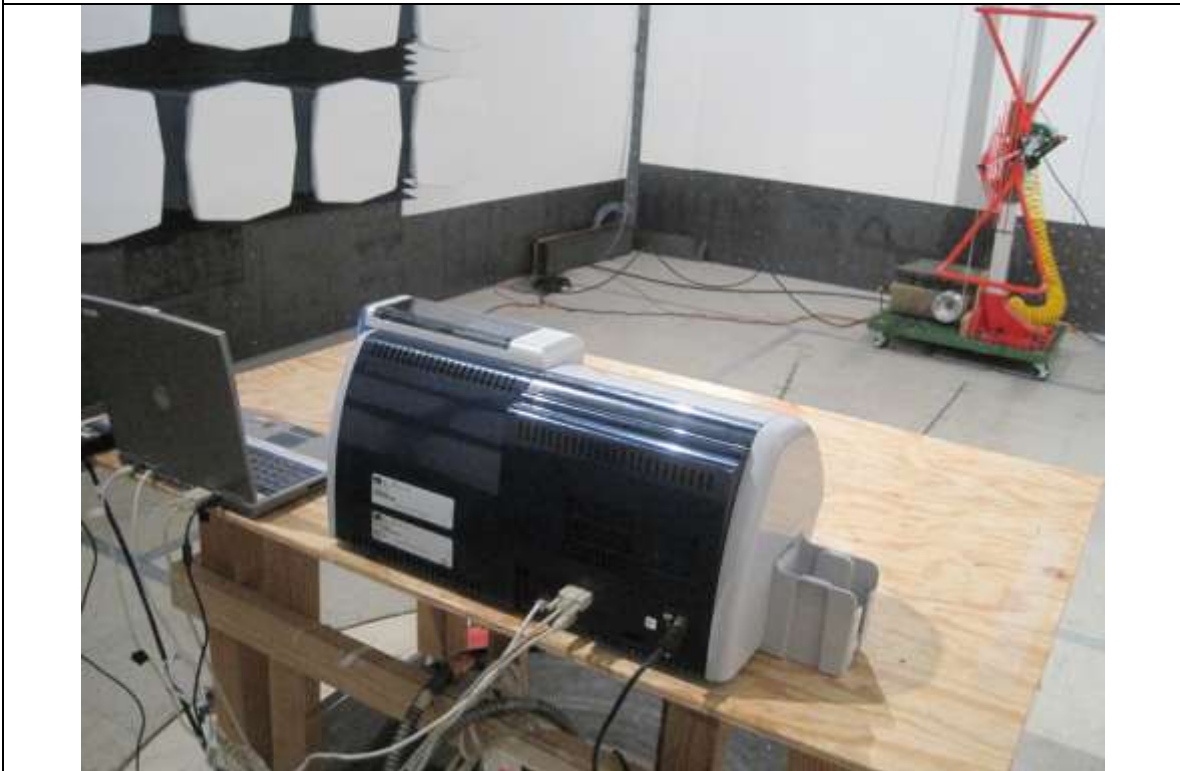
Radiated Emission Test Setup (Above 30MHz) - Rear View
