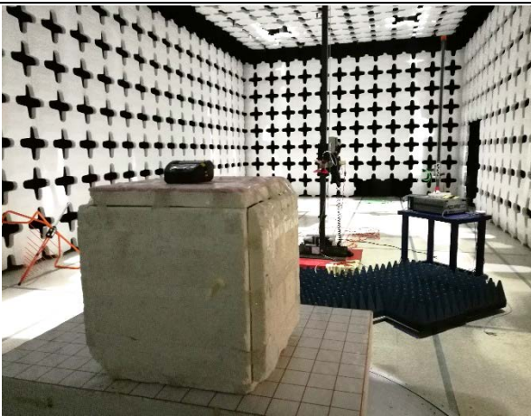
Radiated Emissions (>1GHz) – Rear View
