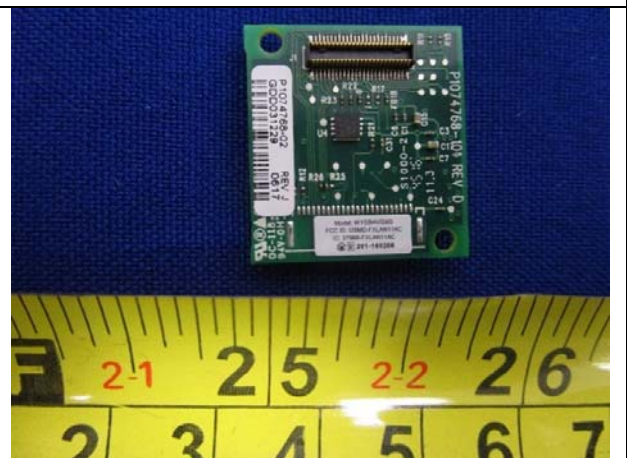
EUT AC Radio Version M/N: ZQ320 P/N: ZQ32-A0W01R0-001 Radio Module – Bottom
