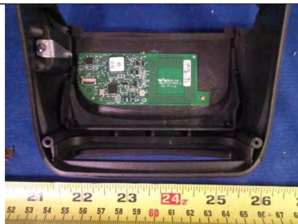
NFC Board Location View
