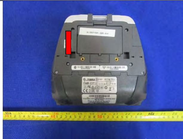
Test Position-1 (Bottom Side with 0mm distance)
